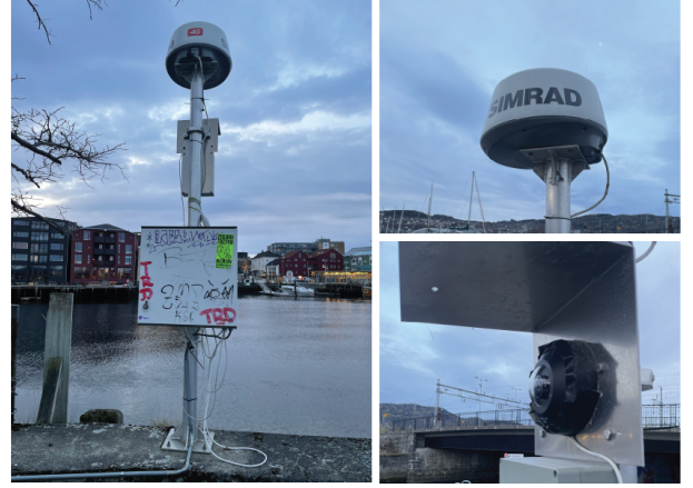
Fig. 1: The sensor station, with a Simrad 4G FMCW solid-state radar and a Sony-Ipela HD SNC-HM662 IP camera.
